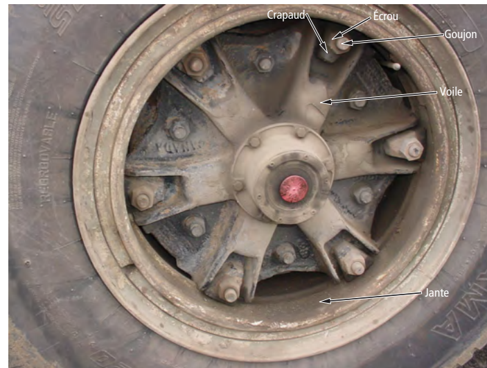
FIGURE 45 | Roue moulée ( spoke wheel )
